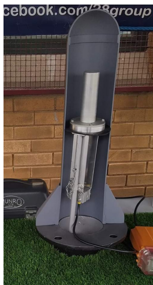
Mike's MAF (Make a Fake) cutaway Fixed Survey Meter Dome shows the PDRM82F sensor.
