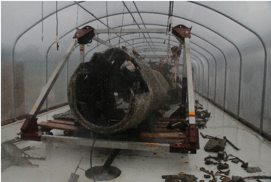
The fuselage of the 'Flying Pencil' in its tunnel being sprayed to remove the salts absorbed during 70 years in the sea.
