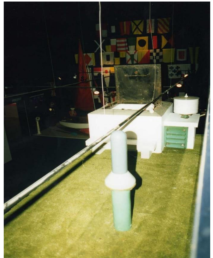
The surface features of the recreated post in the Museum of Lancashire, taken from the viewing gallery; unfortunately the lighting was not good. The FSM dome, hatch and GZI are all visible as is the artificial grass forming the roof of the post. The Sea Cadets display can just be made out in the background. (1993 – copyright John Gedge)
